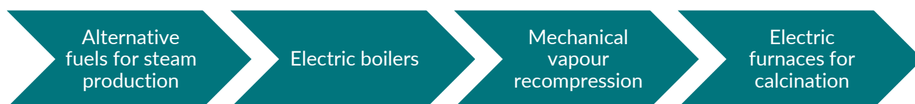
Figure 4. Expected deployment of technologies to reduce emissions from alumina refineries (European Aluminium, 2023)
